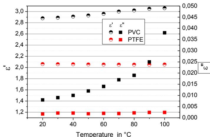
Fig. 6: Complex permittivity measurement for PTFE and PVC as a function of temperature at 2.45 GHz.
