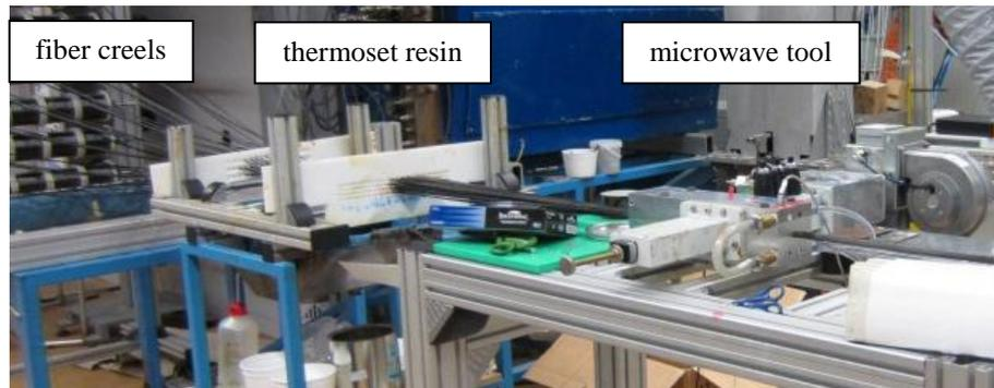
Fig. 4: Picture of a microwave assisted pultrusion experiment.
