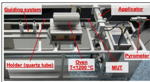
Fig. 7: Set-up for temperature dependent dielectric measurement using the cavity perturbation method.
