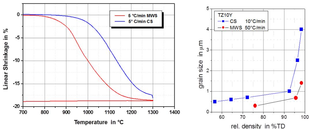
Fig. 2: Comparative studies on mm-wave sintering of yttria-stabilized zirconia. Results of dilatometer experiments (left) [5] and grain size evolution (right) [6].
