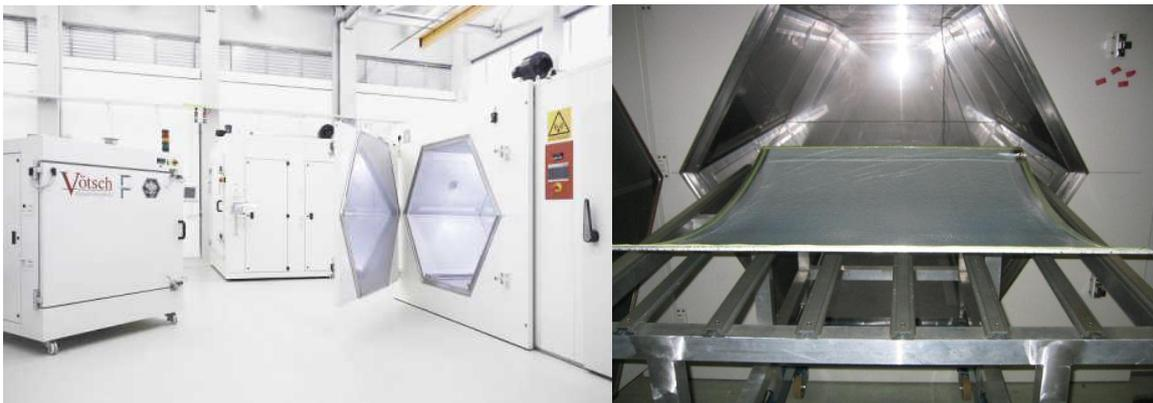
Fig. 3: Photography of the HEPHAISTOS Experimental Center and set-up for a VAP process for CFRP curing.
