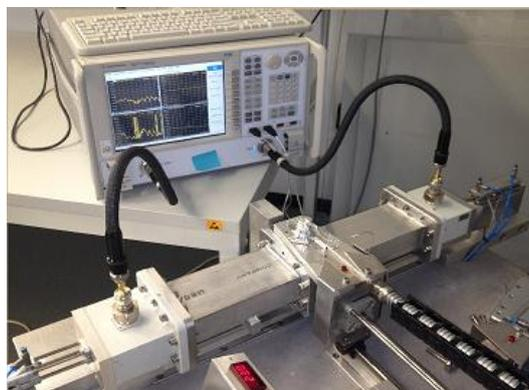
Fig. 5: Set-up for temperature dependent dielectric measurements using transmission-reflection method.
