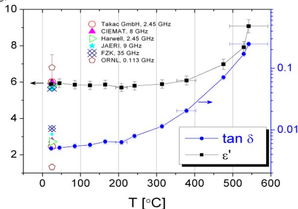
Fig. 8: Dielectric properties for MACOR material. Some previously reported data at roomtemperature are presented for comparison.
