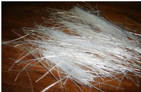
Fig 1. Roving Fiber
