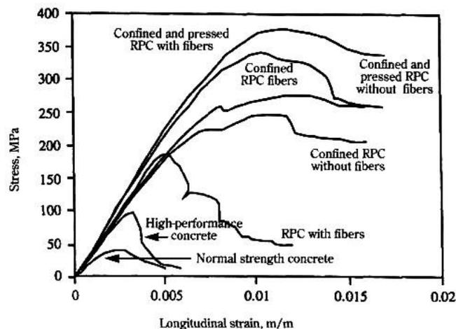
Figure 2. Stress-strain curves of NSC, HSC and RPC, 1998 [10].
