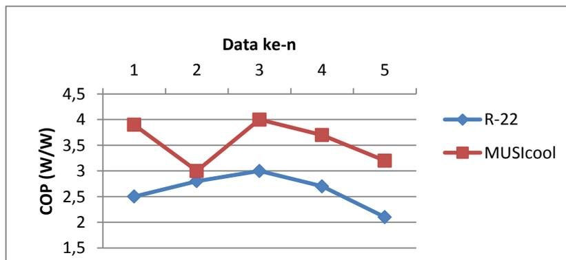
**Figure 3.** Comparison COP data of cold room type A/C 4 kW with R-22 and with MUSIcool at assumed ambient temperatures of 35°C.
