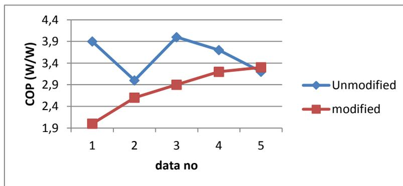
**Figure 4.** Comparison of COP between unmodified and modified inlet diameter of centrifugal compressor with MUSIcool refrigerant and assumed ambient temperature 35°C.
