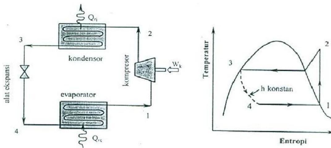
Figure 2.1. vapor compression cycle
