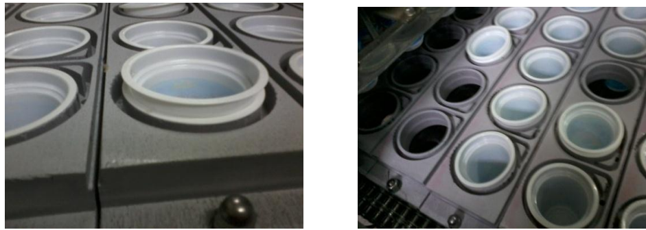
Fig. 10. Cups in bucket of filling drinking machine (influence of electrostatic)
