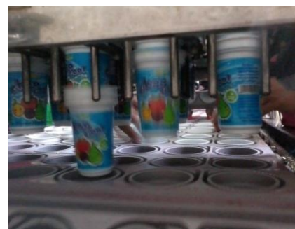
Fig. 8. Pair of cups condition (high electrostatic)
