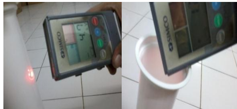
Fig. 3. Measurement of surface electric potential cup by field mill (inner and outer surface)
