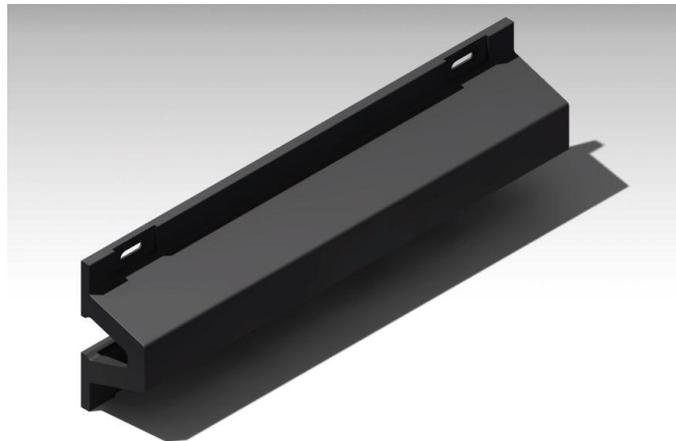
Figure 1. Rubber fender v- type design using Catia V5
