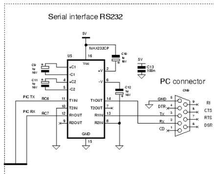
Fig. 6. Development board with a serial connection to/from the PC that lets RS232 work between a microcontroller and the PC
