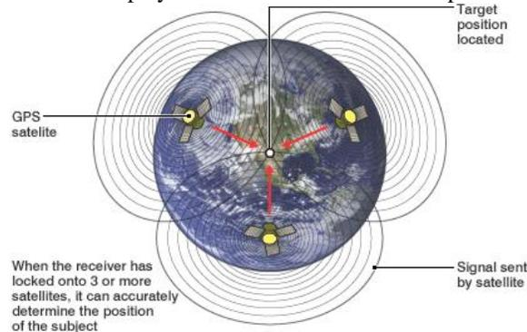
Fig. 7. How GPS with three satellites works
