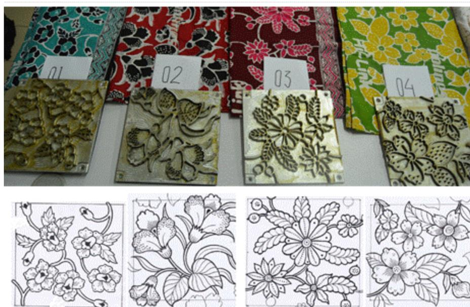
Figure 2. The hand made of batik images (below), the machined batik stamps (middle) and the resulted fabric batiks (top)
