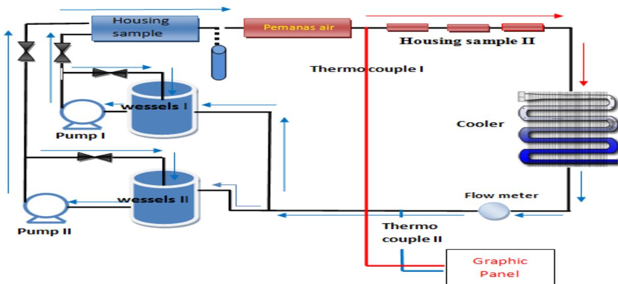
Figure 2. Equipment simulator scale formation unit
