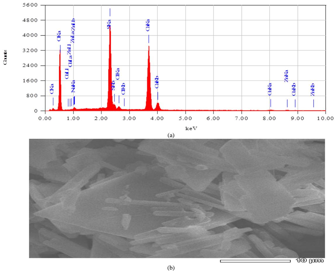
Figure 4. (a) Composition chemistry graph and (b) Morphology of Calcium sulfate
