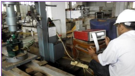
Figure 5. Shear strength bamboo block lamination testing setting-up
