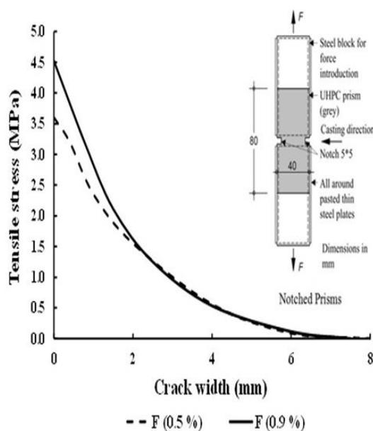
Figure 1. Average stress-crack width diagram [2]
