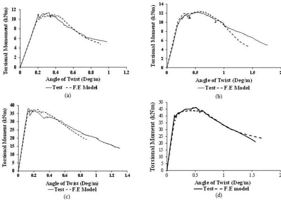
Figure 8. Comparison between test results and F.E prediction for the test beams: a) UPF(0.5)18, b) UPF(0.9)18, c) UPF(0.5)28 and d) UPF(0.9)28 [2]
