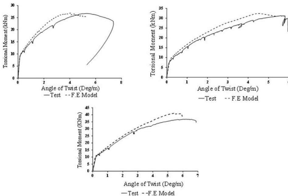
Figure 9. Comparison between test and F.E prediction for the test beams: a) UL(1.4)T(1.96)F(0.5)18, b) UL(2.48)T(1.96)F(0.5)18 and c) UL(2.48)T(2.96)F(0.5)18
