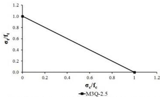
Figure 2. Reduction of tensile strength due to lateral compression [5]
