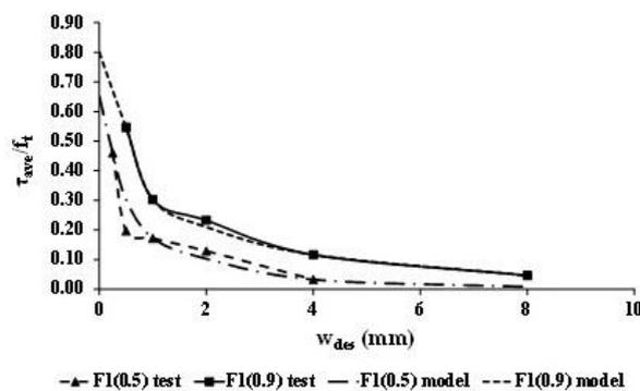
Figure 4. Degradation of the shear strength of UHPC-M3Q with steel fibers due to cracking (test results against proposed model) [2]
