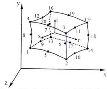
Figure 7 Quadratic isoparametric brick element with 20 nodes
