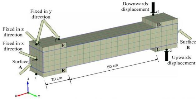
Figure 6 Geometry, loading, supports and mesh of the finite element model of the UHPC test beams [2]
