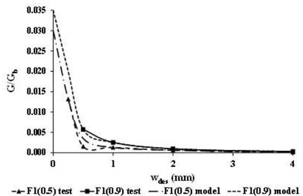
Figure 5. Degradation of the shear stiffness of UHPC-M3Q with steel fibers due to cracking (test results against proposed model) [2]
