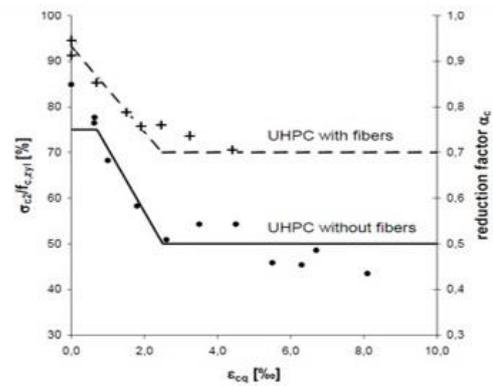
Figure 3. Reduction of the compressive strength of UHPC due lateral tensile strain [6]
