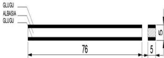
Figure 11. EPA (An adhesive material: glue epoxy, and position wood: albasiah in the middle)
