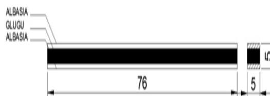
Figure 9. EPG (An adhesive material: glue epoxy, and position wood: glugu in the middle)
