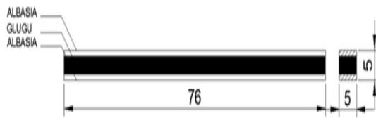
Figure 10. AIG (An adhesive material: glue aibon, and position wood: glugu in the middle)
