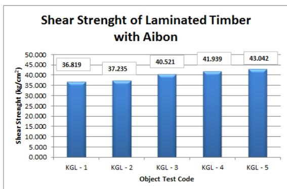
Figure 5. Shear strength of laminated timber with aibon
