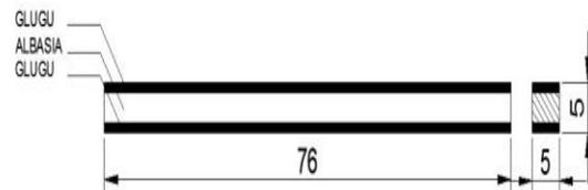
Figure 12. (An adhesive material: glue aibon, and position wood: albasiah in the middle)
