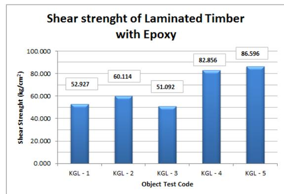
Figure 6. Shear strength of laminated timber with epoxy
