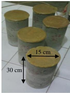
Figure 2. Samples Concrete Cylinder (D15 cm x 30 cm)
