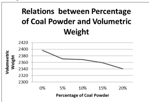
Figure 4. Relations between percentage of coal powder and volumetric
