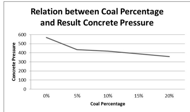
Figure 5. Relations between coal percentage and result concrete pressure
