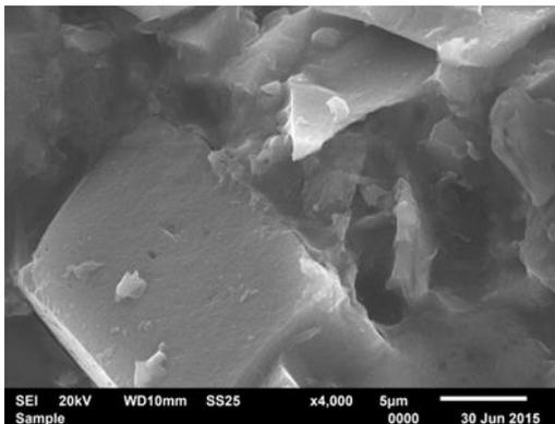
Figure 2. Morphology N – TiO<sub>2</sub> enlarge 400 X
