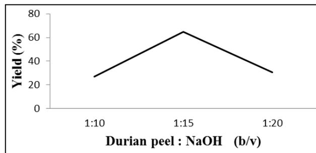
Figure 1. Effect of durian peel Ratio: NaOH to yield of cellulose
