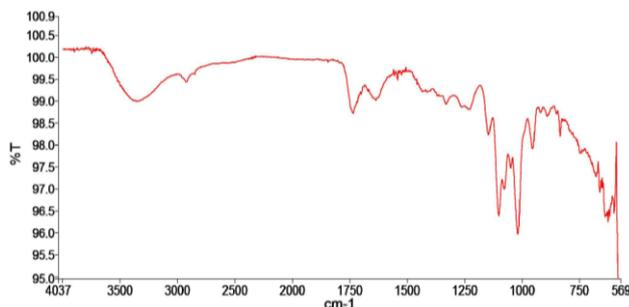
Figure 1. The spectrum of pectin from the balinese orange peel extraction with hydrochloric acid using MAE method
